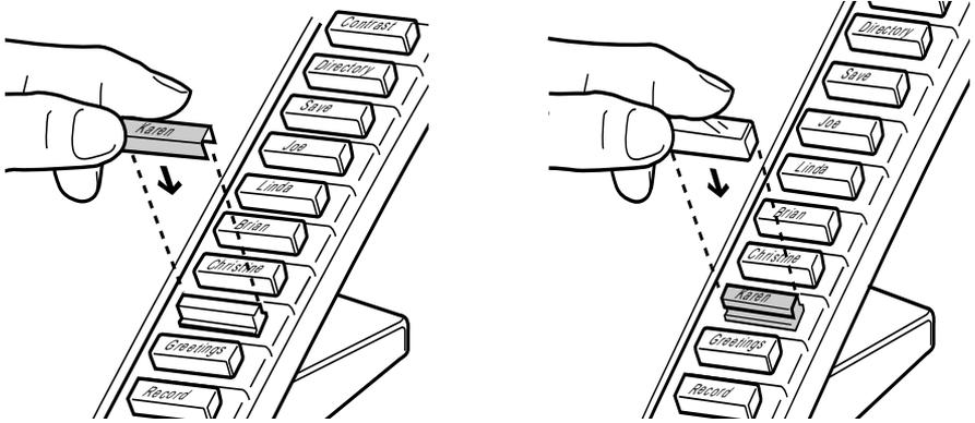
After programming the memory keys, label them with the supplied blank labels and key caps.<sup>†</sup>
