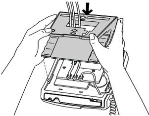
Lower the stand into the slots on the base of the telephone, as shown above.
