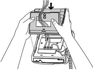
Lower the stand into the slots on the base of the telephone, as shown above.
