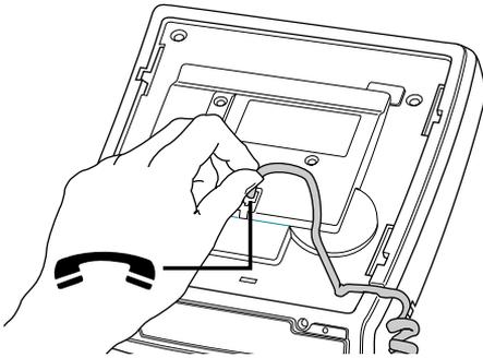
Attach one end of the handset cord to the handset and the other end to the handset jack.
